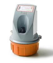
Point Orange 3G is a compact Logger/RTU device with integrated battery, a 3G modem with GPRS fall back, internal and/or external antenna, flexible I/O options, Modbus and SDI-12 master capability and a submersion sensor.
